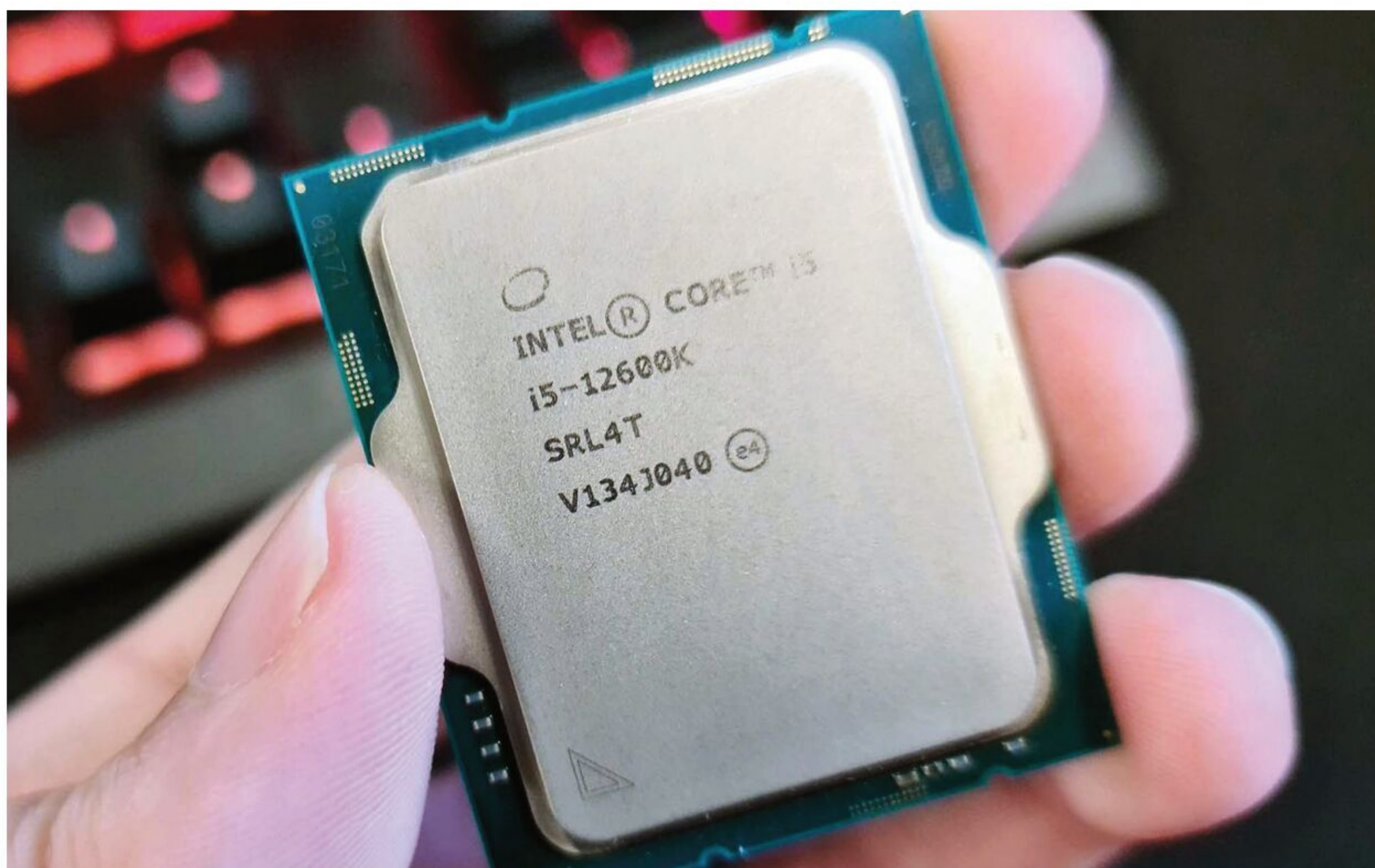
The Intel Core i5 12600K comes with both Performance and Efficient Cores.
